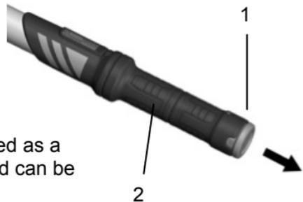
Turn the handle (2) until the desired torque in the particular scale (3) N·m or lbf·ft / lbf·in is identical with the mark in the reading glass.
