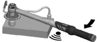
Now set the torque wrench to its max. permissible torque. Set the degree disk to the desired angle.
