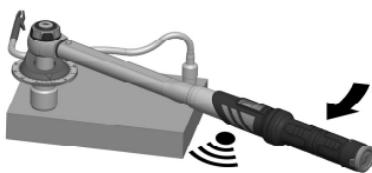
Now set the torque wrench to its max. permissible torque. Set the degree disk to the desired angle.
